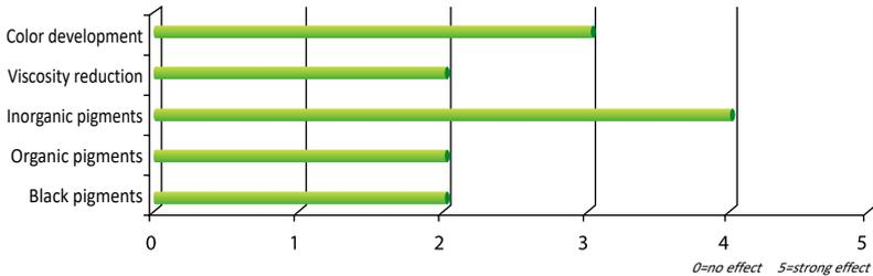
**UNIQ® SPERSE P-160** is a wetting and dispersing additive in unsaturated resin systems and adhesives. The additive prevents the flooding/floating and settling of pigments and fillers in epoxy and VE/UP-based laminates. Reduction in the flooding/floating of colored pigments in gel coats.
