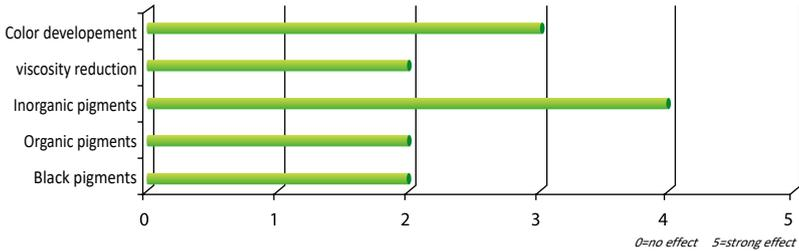
**UNI<sup>Q</sup>® SPERSE P-904** is a wetting and dispersing additive in unsaturated resin systems and adhesives. It's no silicone dispersant. The additive prevents the flooding/floating and settling of pigments and fillers in epoxy and VE/UP-based laminates. Reduction in the flooding/floating of colored pigments in gel coats. And it can reinforce the rheological effectiveness of pyrogenic silica to increase and stabilize the thixotropic behavior.
