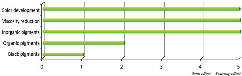
**UNIQ® SPERSE P-193** is a wetting and dispersing additive for filled unsaturated polyester, epoxy systems, PVS plastisols and thermoplastic applications. The dispersant is especially suitable for inorganic pigments and filler pigments. Strong viscosities reduction so higher pigment and filler loading in the grinding process can be achieved.
