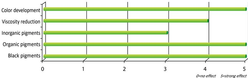
**UNIQ<sup>®</sup> SPERSE P-172** is a wetting and dispersing additive for inorganic pigments, organic pigments and carbon black in adhesive, plastisols, ambient curing resin systems, and for the production of color pastes for thermoplastics. It is also very suitable for SMC/BMC and pultrusion to homogenize and stabilize the system, and to increase the color homogeneity in molding compounds; and it can give good fiber wetting and anti-separation performance.
