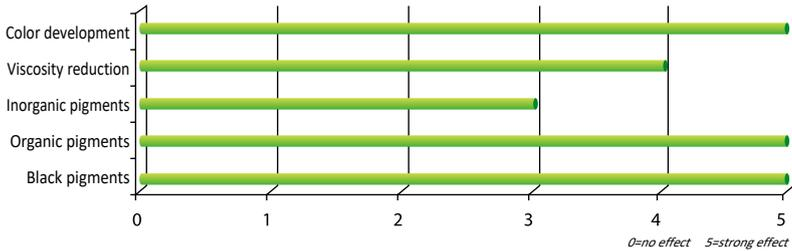
**UNIQ<sup>®</sup> SPERSE P-185** is a solvent-free wetting and dispersing additive, very suitable for solvent-borne and solvent-free adhesives, PVC plastisols, ambient curing resin systems, and for the production of color masterbatches for thermoplastics. Particularly recommended for organic pigments, inorganic pigments and carbon black. And it's also suitable for epoxy flooring system.
