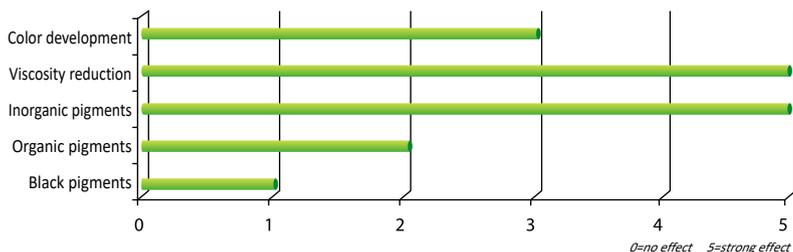
**UNIQ<sup>®</sup> SPERSE P-195** is a wetting and dispersing additive for filled unsaturated polyester. The dispersant is especially suitable for inorganic pigments and filler pigments. Strong viscosities reduction so higher pigment and filler loading in the grinding process can be achieved.
